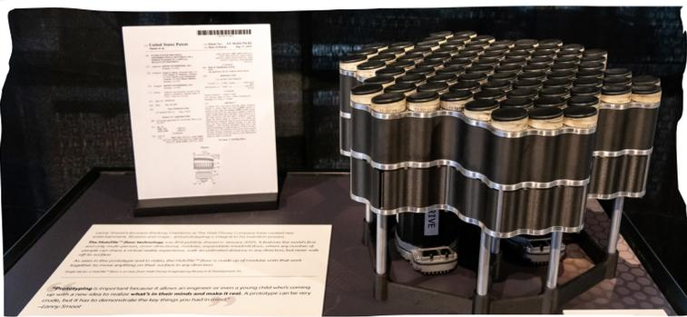
A new exhibit allowed visitors to see a prototype of HoloTile™ floor technology, co-created by 2024 Inductee Lanny Smoot, The Walt Disney Company's most prolific inventor. The HoloTile floor is the world's first and only multi-person, omni-directional, modular, expandable treadmill floor.
