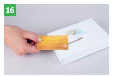
Tap the card on top of the conductive tape on the box. Apply pressure to get the LED to light up!
