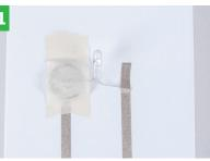
Place the other lead of the LED on top of the coin battery. Tape into place.
