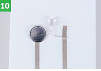
Place a coin battery, with the negative side up, on top of the tape.
