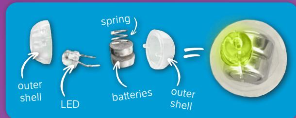
Congratulations! You've unlocked your LED ball! Check out the inner parts that make the LED ball's circuit!
