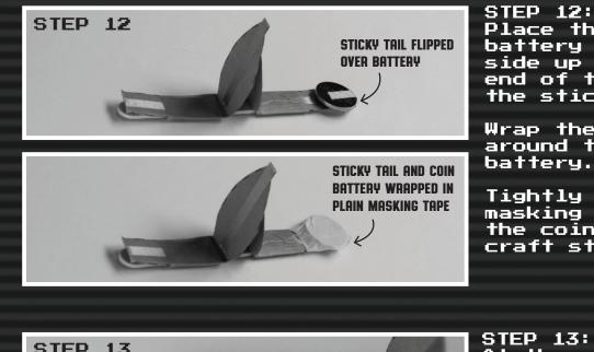
Place the coin battery + (positive) side up at the end of the stem near the sticky tail.
