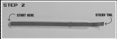
STEP 2: Remove the backing from the conductive tape. Starting at one end, stick the tape along the craft stick. Leave a sticky tail hanging off the end.
